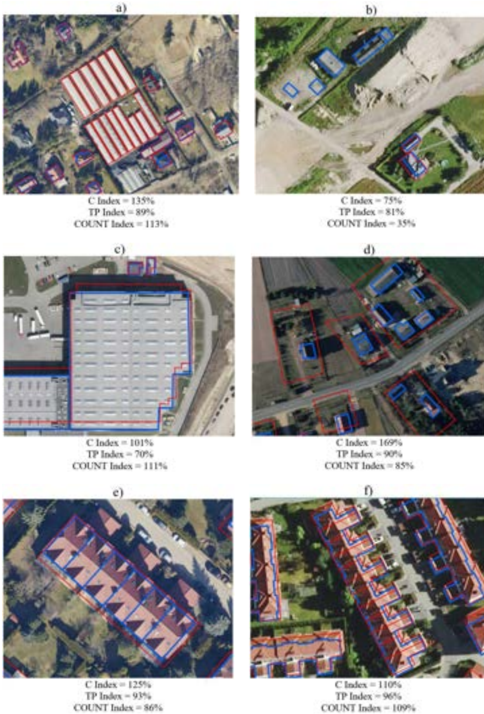
Fig. 6. Comparison of the analyzed buildings location from the OSM database (red) and BDOT10k (blue) on the orthophotomap, along with the values of the calculated completeness indices: C Index, TP Index, COUNT Index
