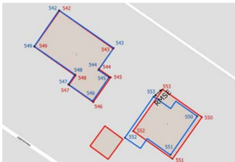
Figure 5. Homologous points semi-automatically detected between the OSM buildings (red) and the BDOT10k buildings (blue).
