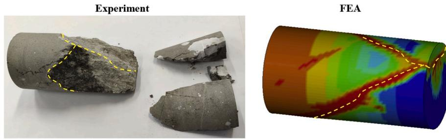
Fig. 12. Comparison of the fracture patterns for TXC 25.0 MPa from simulation and experiment.
