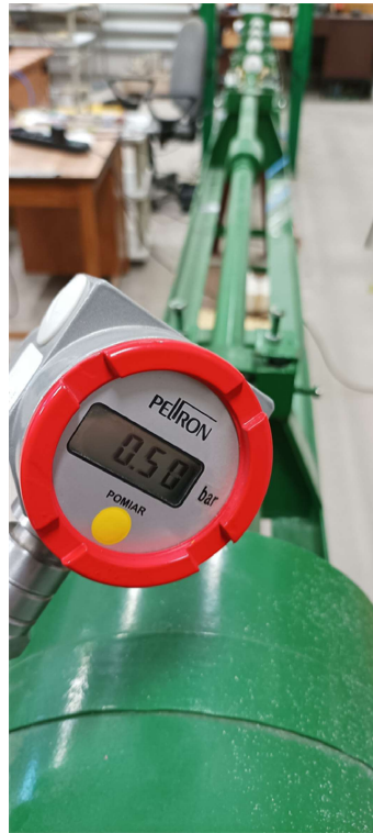
Figure 2. The value of the pressure given by the pneumatic launcher for the shot - initial compaction of the soil sample
