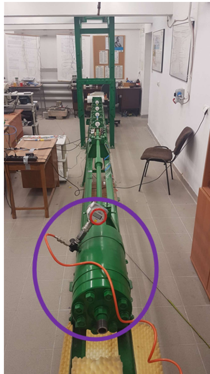
Figure 8. View of the pneumatic launcher (purple marking) as an important element of the SHPB test stand.
