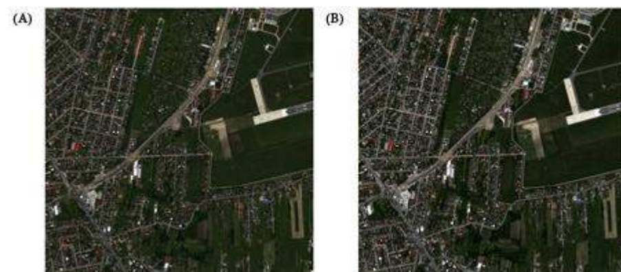
Figure 9. Sample test image—fragment of a multi-spectral image captured by the World View-2 satellite, depicting the suburbs of the town of Radom: (A) low-resolution (LR) image (dimensions: 917 \times 921 pixels), (B) high-resolution (reference) image obtained as a result of pansharpening with the Gram–Schmidt method (dimensions: 3667 \times 3684 pixels).
