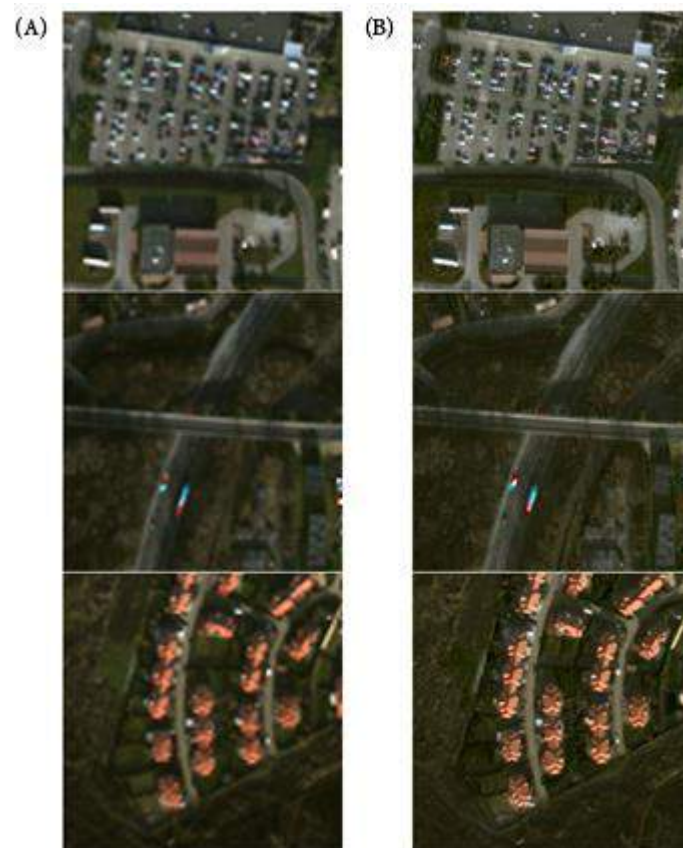
Figure 6. Sample pairs of (A) LR and (B) HR images that were used to train the ESRGAN network.
