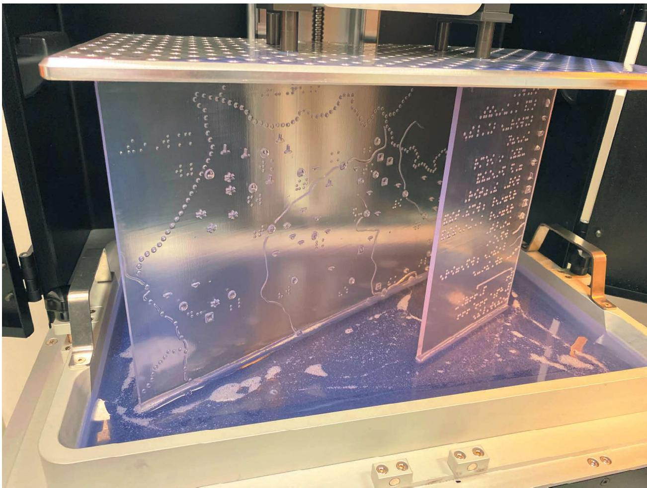
**Figure 13.** The stereolithography printing process using transparent resin.
