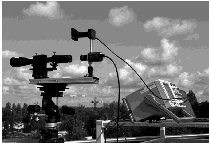
Fig. 65. Measuring device: Si Photodiode with a UV filter (upper) with visible sight camera (lower)
